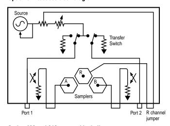
Option 400 and 012 test set block diagram
