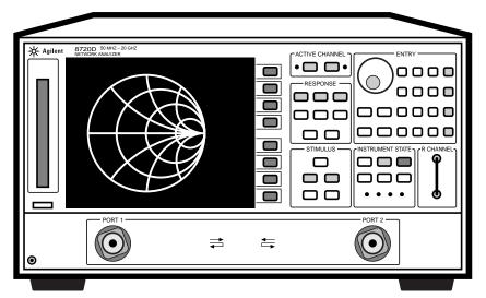
8719D 50 MHz to 13.5 GHz 8720D 50 MHz to 20 GHz 8722D 50 MHz to 40 GHz
